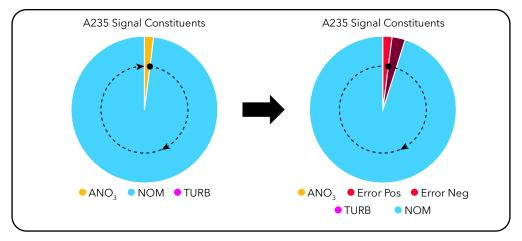
In this case, with the same +5% overestimate for the NOM coefficient, the nitrate estimate is now consumed by the error resulting in negative NitraLED readings.
