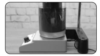
Set up the stir plate under a ring stand or other device that will hold the EXO during this procedure. Place a 1 L beaker on the stir plate and fill to approximately 800 mL with raw sample water. Place the stir bar in the sample water. Turn the stir plate on to a speed slightly higher than that of the site environment that keeps all sediments suspended as they would be in the natural water body.
