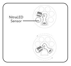
(Top view) Center Wiper Arm within NitraLED Sensor window
