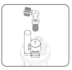
Slide Brush down until fully seated on top of the Central Wiper
