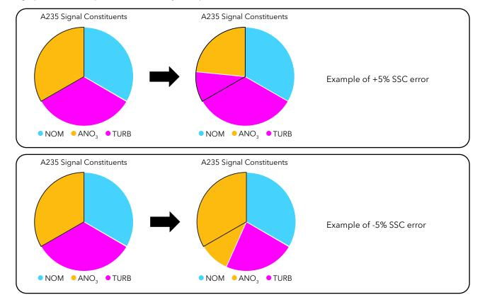
With a positive 5% error in the SSC coefficients, the effect of turbidity and NOM interference is overestimated, resulting in an underestimation of nitrate. With a negative 5% error in the SSC coefficients, nitrate is overestimated.
