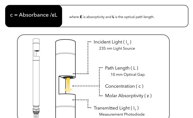
The concentration of nitrate ions,  $NO_3^-$  mg/L, is proportional to the optical absorbance of the UV-C radiation. It is important to note, however, that the UV method presented by YSI does not distinguish between nitrate  $NO_3^-$  and nitrite,  $NO_2^-$ , owing to similar UV absorption properties and we therefore denote the combined species,  $NO_3^-N$  (nitrate as nitrogen). However, in natural waters, nitrate is typically the most prevalent species.
