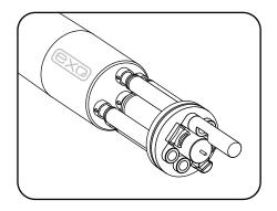
Once the o-ring is fully seated around the Alignment Ring, installation is complete.
